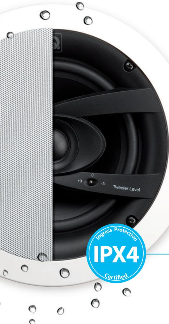
The IP Code, International Protection Marking, IPX4 classifies and rates the degree of protection provided against the intrusion of moisture, such that water splashing against the enclosure from any direction shall have no harmful effect
